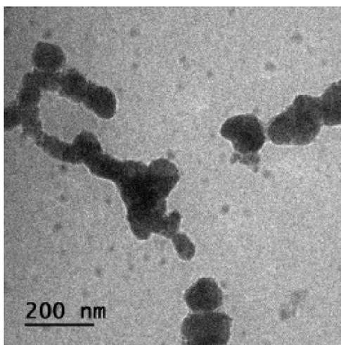
Nano-particles in the photoresist
